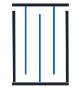
Biogas frame of plate heat exchanger (R-171). Biogas inlet left. Syngas outlet right. Frame in black. Baffles in blue.
