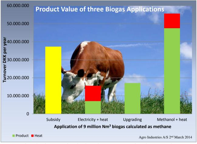
Biomethanol value exceeds subsidy making it a most robust biogas application.
